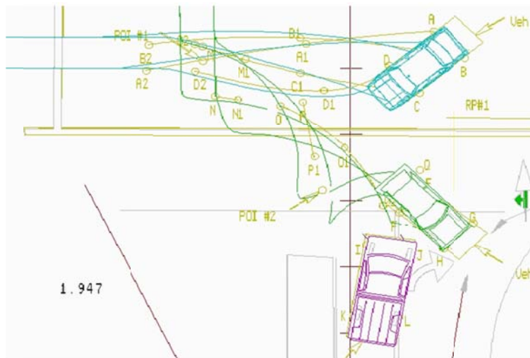
Figure 15 Sample of SMAC Collision Reconstruction
